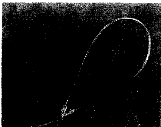
Fig.3 A microdialysis probe for subcutaneous continuous measurement of glucose.
